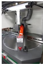
The IRONWOOD CUT20M up-cut saw offers operators a safe and reliable, compact crosscutting solution with a rotary table for miter cuts. The table surface of the CUT20M is precision-ground to ensure absolute cutting accuracy while maintaining maximum stability during heavy cutting operations. The pneumatically-operated machine highlights enhanced safety guards, fast cutting speeds, and the powerful motor torque required when working with multiple material types and dimensions.
