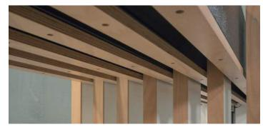
**Pressing surfaces with tolerance compensation**: The pressing lamellas work as a unit; they are placed on rubbers and suspended. Pressure is very evenly distributed due to the fact that the pressing lamellas simultaneously impinge on the carcass.
