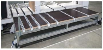
**Movable pre-plugging station**: The pre-plugging station allows a simple assembly of the carcasses at working height of the press.
