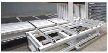
**Manuel carcass erecting device**: The carcass erector is used for erecting and transporting mounted carcasses.
