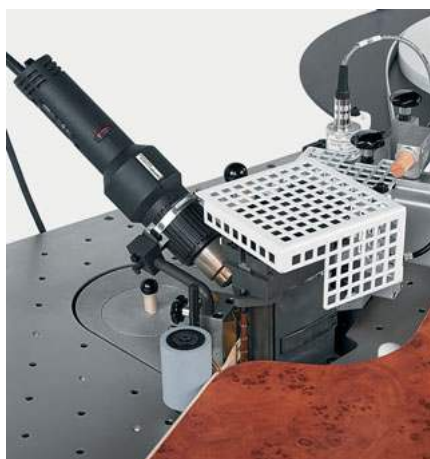
Additional heating unit (optional) To pre-heat thick PVC-edges.
