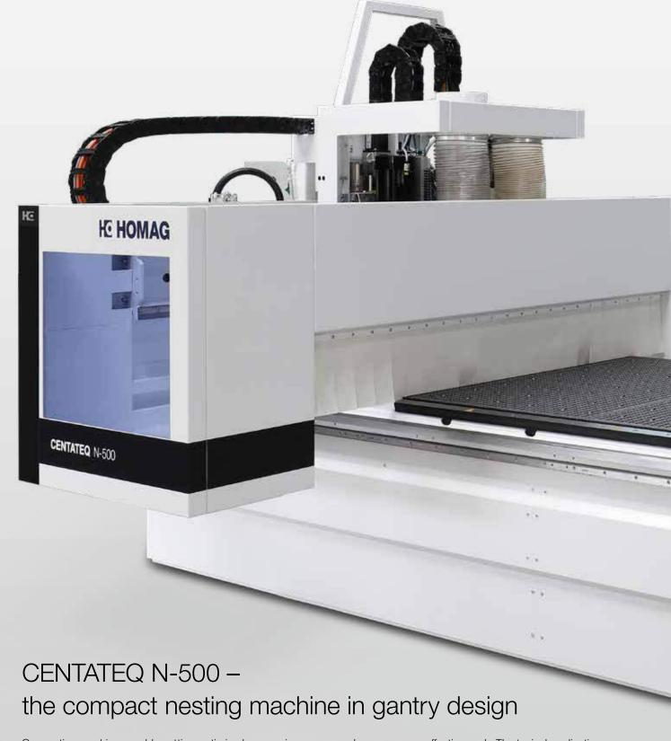
Our nesting machines enable cutting-optimized processing and dividing of plateshaped materials. We divide the typical nesting areas into four areas. Various possibilities for the automation of the material handling ensure a high time saving and an even more effective work. The typical application areas of nesting: Creating components for carcass furniture, dividing and refining of furniture fronts and processing of frame.
