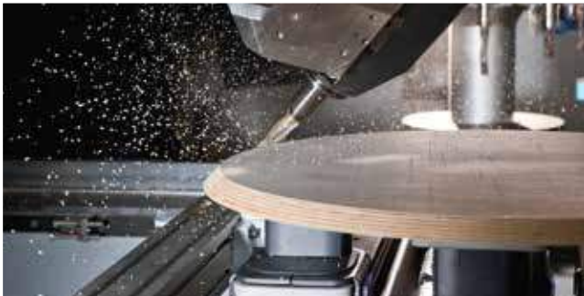
Chamfer trimming on a table top
