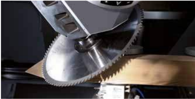
Mitre cut with high cutting depth for frames
