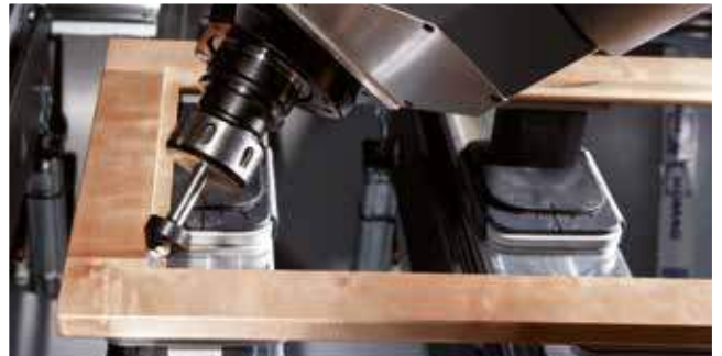
Square corner routing for a glass rebate
