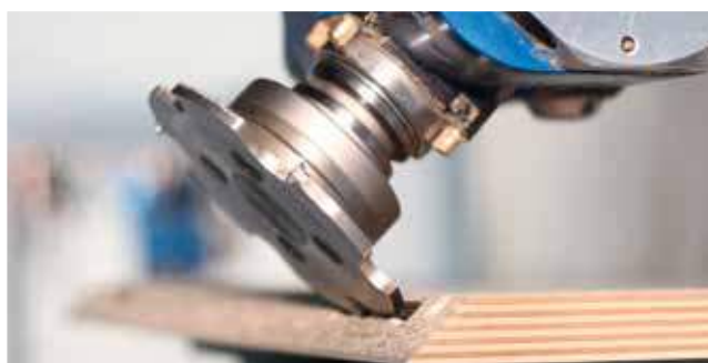
Cutting recesses for connecting fittings
