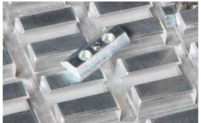
Slot nuts with thread for positive locking of clamping fixtures in the dovetail guide
