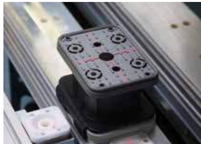
LASER positioning aid – vacuum suction units are indicated by a laser cross-hair. The workpiece contour can be “moved” as a positioning aid for free-formed workpieces.
