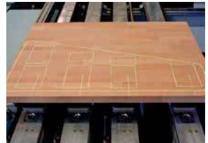
Laser projection of the clamping equipment and the workpiece contour for optimal utilization and simple positioning of unprocessed parts that cannot be aligned on the stops.
