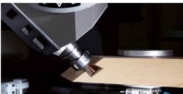
Routing of a dovetail joint for upright / transom constructions
