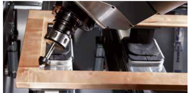
Square corner cutting for a glass rebate
