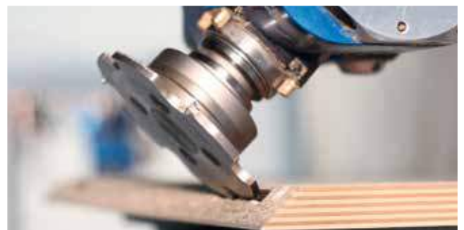
Cutting recesses for connecting fittings
