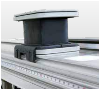
Measuring tape for positioning the suction units.
