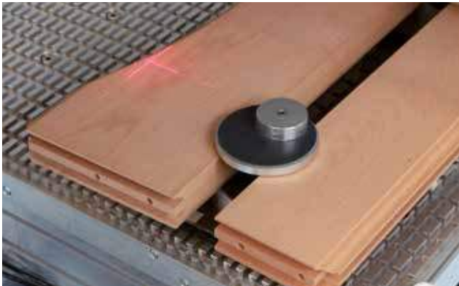
Laser positioning Routing contours can be processed via the cross-laser
