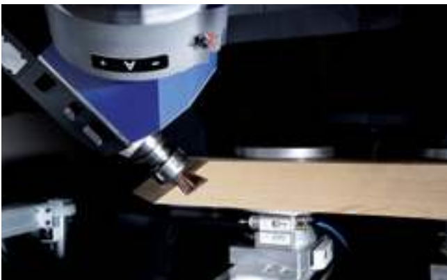
Routing a burr connection for jamb/rail designs
