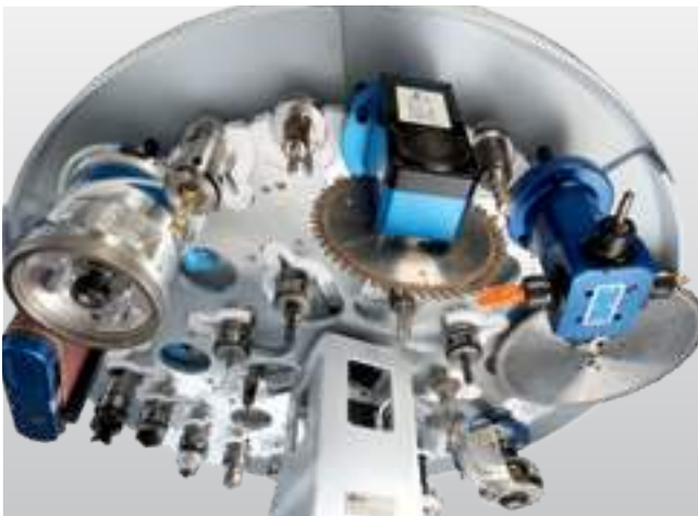
32-space tool changer – arrangement of the tools in an inner and an outer ring. For tools and units with a diameter of up to 200 mm and saw blade up to 350 mm in diameter (in the outer ring).
