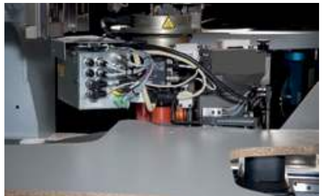
360° edge gluing with the powerEdge edge banding unit
