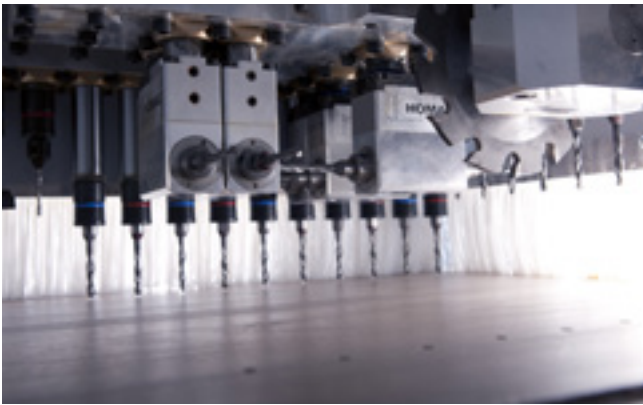
High-speed drilling technology with groove saw
