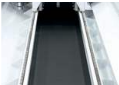
Chip conveyor for easy disposal of the offcuts and chips.
