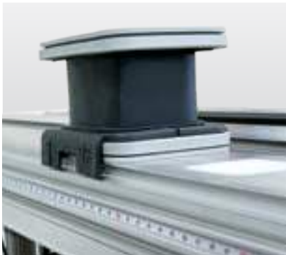
Measuring tape for positioning the suction units.
