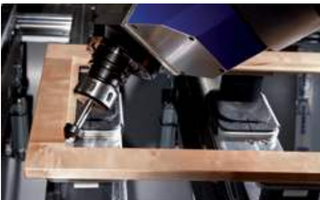
Angular cutting of a glass rabbet corner
