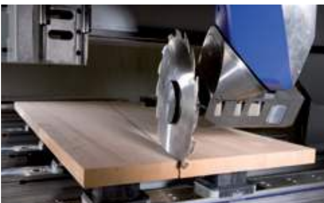
Separating cuts up to 110 mm in height
