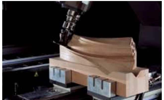
Routing a staircase handrail
