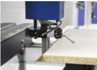
Scraping of mitered edges
