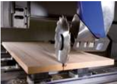
Dividing cuts up to 110 mm in height
