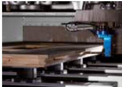
Lock case trimming on front doors
