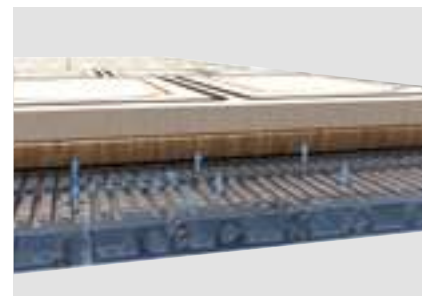
Vacuum grid table with air cushion function: The vacuum transmission is integrated in the design of the aluminium grid table. Division into zones and efficient vacuum pumps ensure reliable clamping, even for nesting processes with underlay panels. The air cushion function makes light work of handling large-format panel-shaped workpieces.
