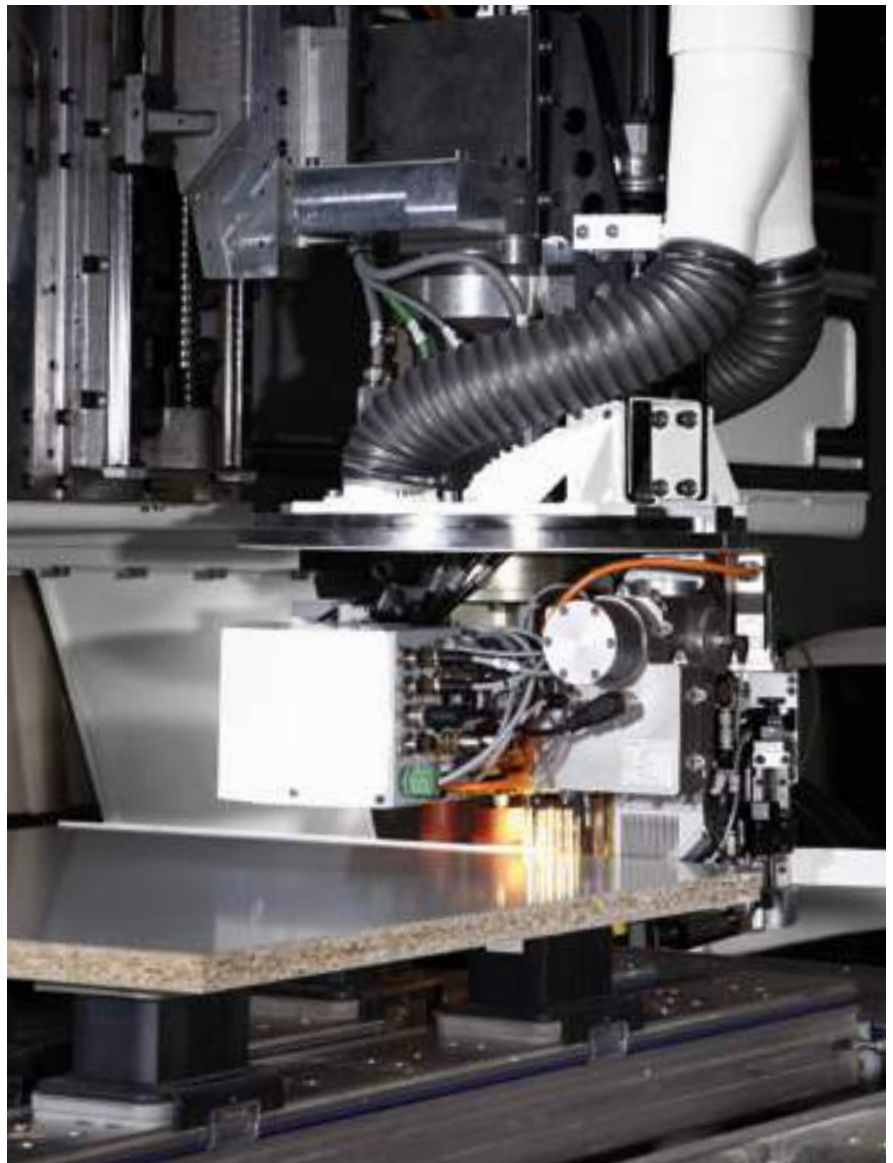
laserTec shaped component edging with zero joint
