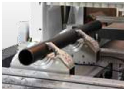
Clamping fixture for round pipes: Clamping fixture for 5-axis processing of round plastic pipes.
