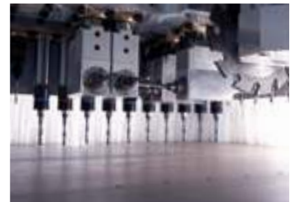
High-speed drilling technology with grooving saw
