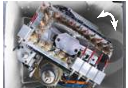
Multi Processing Unit (MPU): The Multi Processing Unit has a stepless 360° swivel action. This allows the saw and also all 20 vertical and 10 horizontal spindles to be applied at any optional angle. An optional trimming spindle attachment saves tool changes and enhances productivity.
