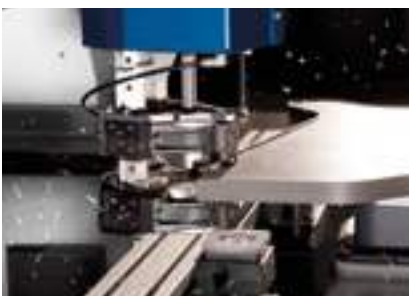
Perfect edge finish with traced combination flush trimming / scraping unit
