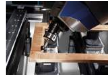
Square corner routing for a glass rebate
