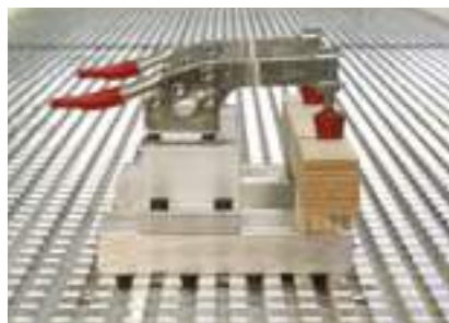
Fixture using non-standard clamps: The aluminium grid table with dovetail guides guarantees precise, positive fitting clamping element fixture.
