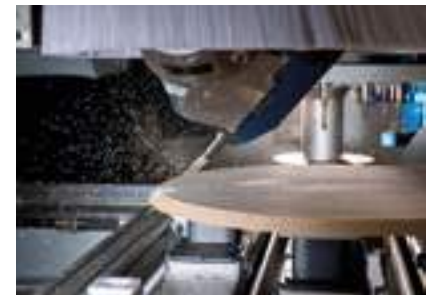
Chamfer trimming on a table top
