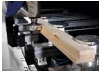
Profiling of frame components
