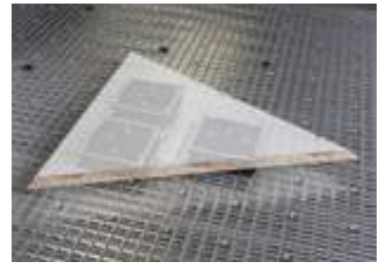
Vacuum clamp: Vacuum clamping elements for insertion in the grooves of the grid table.
