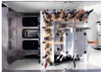
Drilling head V12/H4: HIGH-SPEED drilling head up to 7500 rpm with 12 vertical spindles, grooving saw and 4 horizontal spindles with 0/90° swivel facility. Fast drilling including grooving in the X/Y direction.
