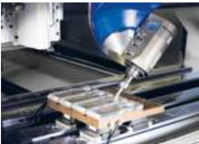
High-gloss trimming of acrylic parts
