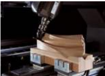
Routing of a stair hand rail
