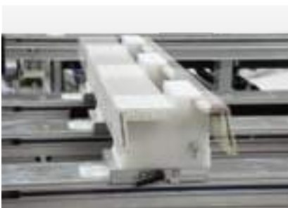
Clamping fixture for facings: Vacuum clamping fixture for a pair comprising rebate and ornamental facings according to customer design. Mounted on a base plate module.
