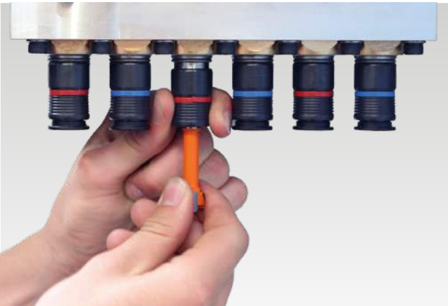
Patented quick-change system for a drill change without tools to reduce setup times.
