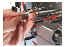
**Drill quick-change system** – The patented system ensures easy installation or change of drilling bits
