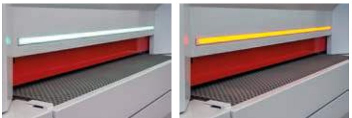
The status of the machine is also displayed via the LED strips in the infeed and outfeed of the machine so that its status is always visible even from a greater distance.
