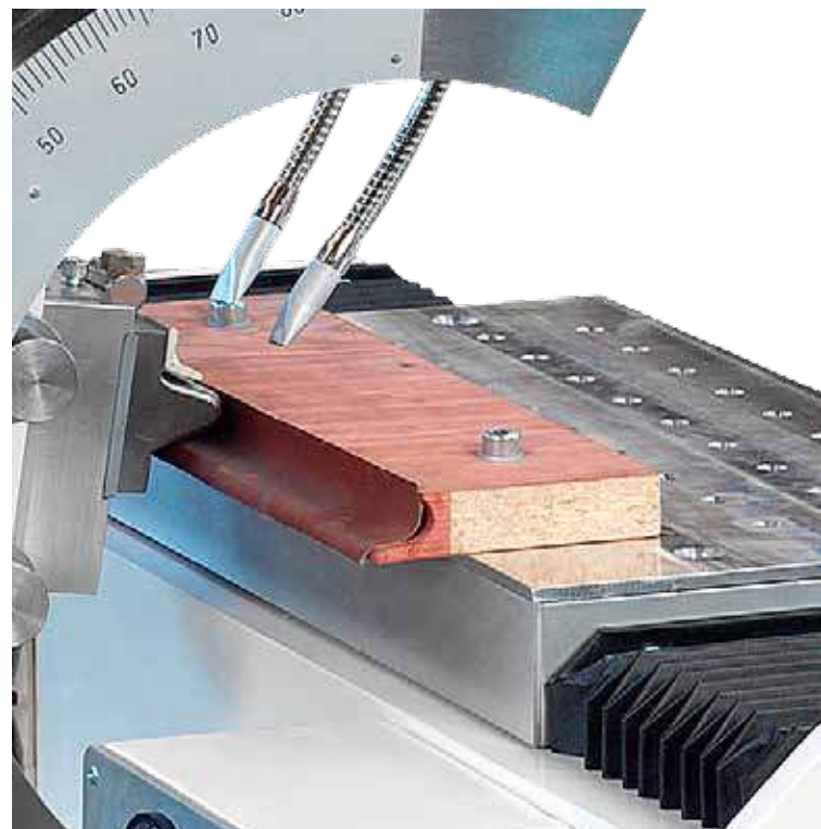
A metal counter profile is made on the PWS-T using a sample work piece.
