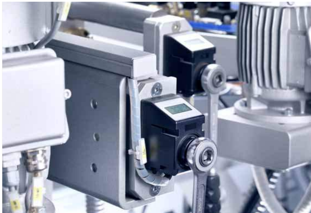
Electronical position indicators connected with the machine control unit allow a comparison of the target value and the actual value of an axis.
