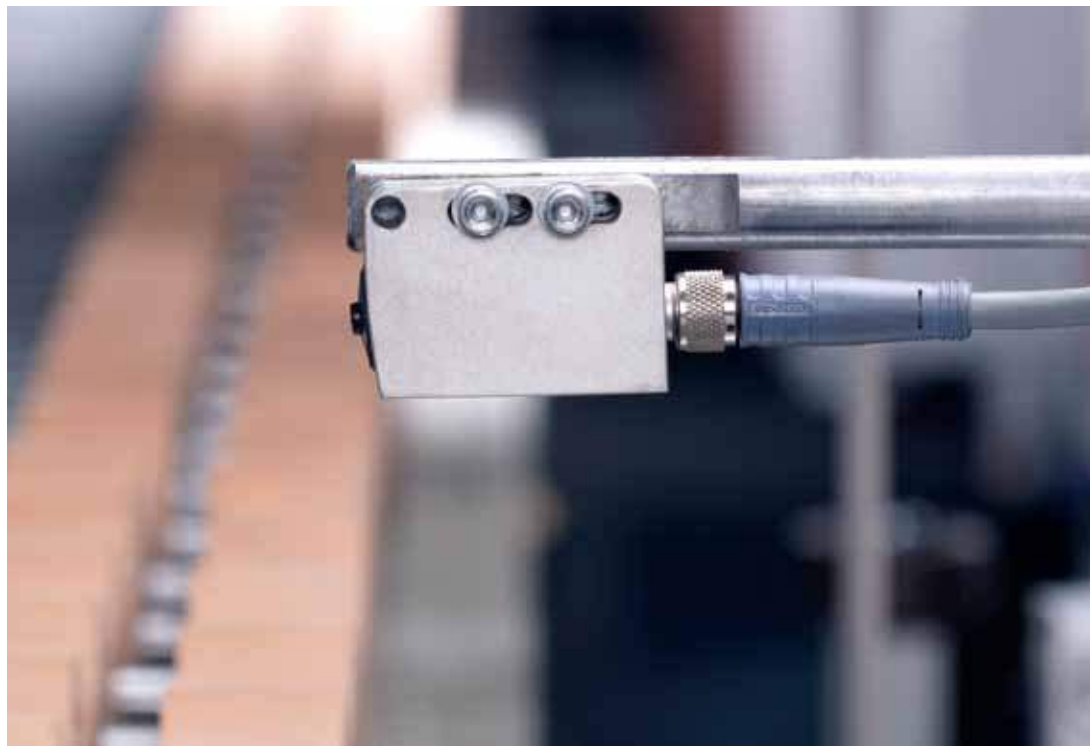
The work pieces are detected at the infeed of the machine.
