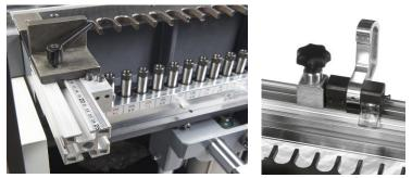
The IRONWOOD BR23 construction Boring machine provides a 23-spindle universal drilling solution, with horizontal and vertical boring capabilities and a fully automated pneumatic tilting of the boring unit from 0 to 90 degrees.
