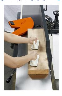
The IRONWOOD JT300 Jointer marks the beginning of fine craftsmanship. This machine offers a 12" cutting width, enhanced engineering designs and superior build construction for long-lasting and trouble-free performance. The JT300 Jointer also includes convenient standards like the interchangeable fold-away bridge guard, a helical cutting system for smooth, quiet operations, and an 84" cutting length.
