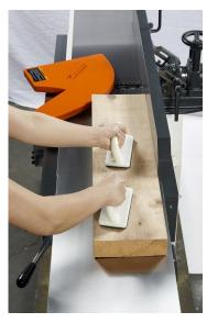
The IRONWOOD JT400 Jointer marks the beginning of fine craftsmanship. This machine offers a 16" cutting width, enhanced engineering designs and superior build construction for long-lasting and trouble-free performance. The JT400 Jointer also includes convenient standards like the interchangeable fold-away bridge guard, a helical cutting system for smooth, quiet operations, and a 96" cutting length.
