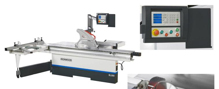
IRONWOOD's SL Series of sliding table saws bring ultimate versatility and flexibility to an operator friendly cutting solution. Fused to be a blend of innovation, dependability and quality, the SL series delivers the quality and precision required for the final chip-free cut, improving the results of subsequent machining.
