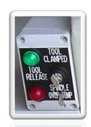
•Simple key switch activated tool release.
