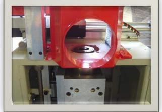
265 DD - HSK uses a 10HP - 18 HP HSK- 63F quick change spindle
