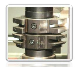
•265-2 Option on the Belt-Drive Version offers a simple, quick and repeatable way to switch from one profile to a second profile in seconds using a pneumatic cylinder and two adjustable stops.
