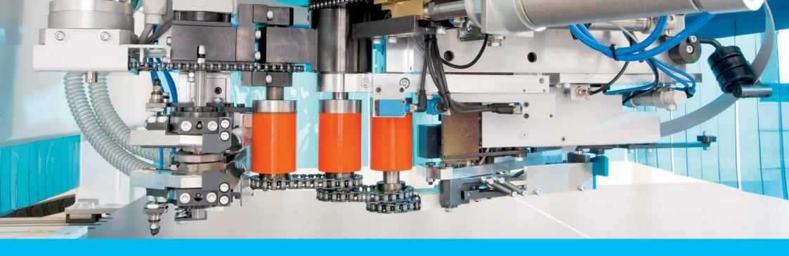
The VECTOR Revolution 180 literally turns contour edgebanding on its head and represents the first significant development of machinery in the composite board industry since the development of CNC machining centres some 20 years ago, broadening the scope for these products beyond rectangular panels.
