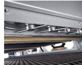
Rotary Air Jet Part Cleaning
