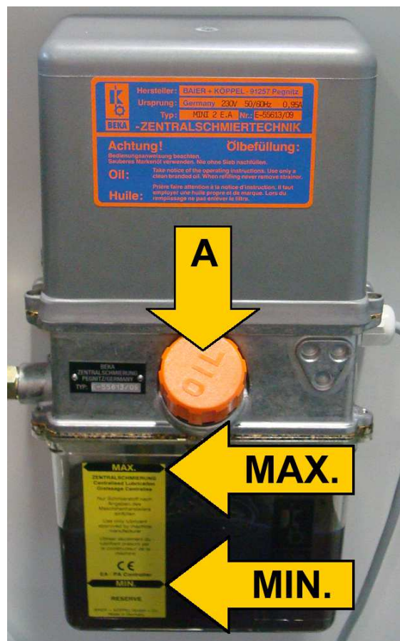
Abb.44 – Central lubrication of the axle drives
