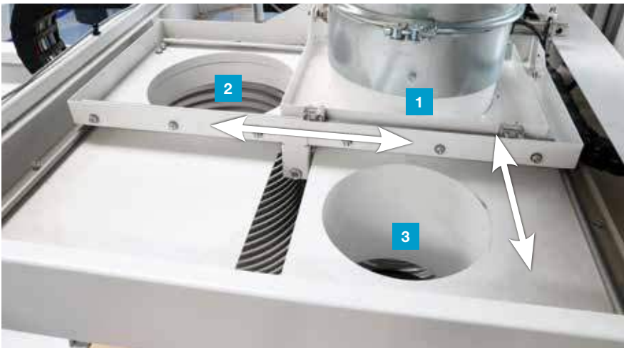
1 Position for the routing spindle 3 Position for the push-off device with integrated suction unit 2 Position for the drilling gear
