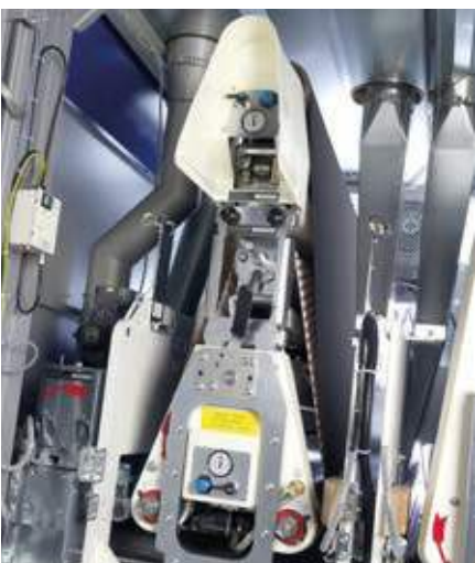
Longitudinal sanding unit (with pressure segment belt)
