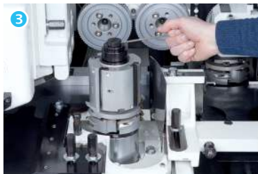
Quick and Easy Tool Change with proven proLock tool clamping system
