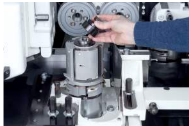
Quick and Easy Tool Change with proven proLock tool clamping system
