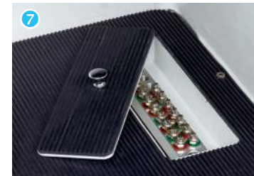
Accessible Central Lubrication at machine front
