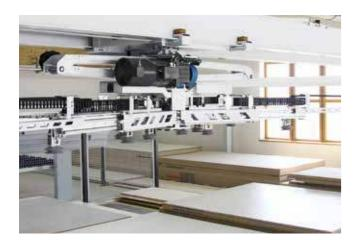
The ST71 suction cross rail in X geometry is the ideal optional feature for the panel storage. The self-learning cross rail generates the data required for panel handling independently and thus ensures dependable process reliability. The operator does not have to enter anything.
