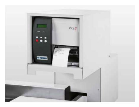
The label printer from HOMAG allows you to print customized labels directly at the saw and design them to include bar codes, text and graphics if required. If you also use our Cut Rite optimization software, the material goes directly to the next process step with printed instructions. In this way, you can integrate the saw perfectly in your production flow.
