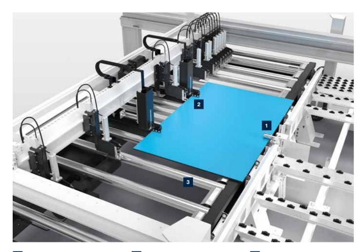
Hold-back device for thin panels (for lifting-table saws and angular saw units only)
