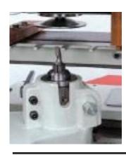
Employs a special collet chuck for absolute centric clamping of the dovetail shank.
