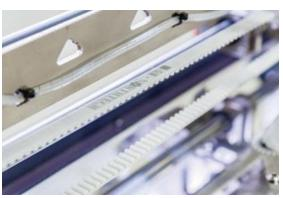
• Precision timing belt mated with servo positioning helps provide the exacting glue placement.
