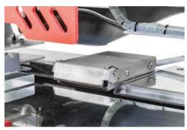
• Rear mounted pressure plate detects part into and initiates cycle automatically.
