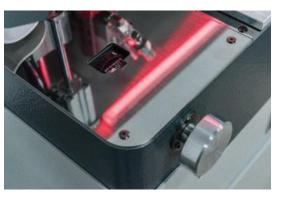
• Board depth placement control via front mounted siko positioning with mechanical readout.
