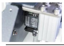
• Servo powered head positioning.
