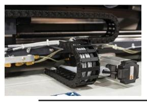
• Pneumatic lines and electrical wiring are encased in industrial cable track.
