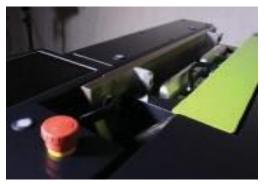
• Outside the touchscreen only (3) physical buttons for a streamline operation; Emergency stop and clamp operation buttons.
