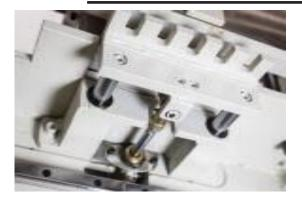
• (2) Auto retracting positioning shelves mounted on dual linear shafts ensure a precise part position.
