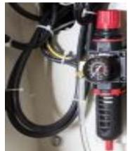
• Regulator, filter and primary shut off value for easy pneumatic connection.
