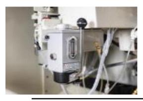
• Central pump lubrication system keeps slide wear points easily lubricated.
