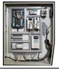
• All electrics are installed in a centralized cabinet for dust free operations and protected inside the body of the dovetailer.
