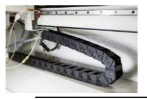
• Pneumatic lines and electrical wiring are encased in industrial cable track.
