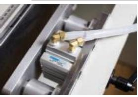
• Both vertical part clamps are bi-directionally powered for quicker part change.
