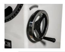
· Quick adjust hand wheel allows for fast blade height adjustments
