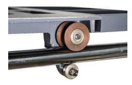
Lineal round rod movements assist with smooth movements during cutting.
