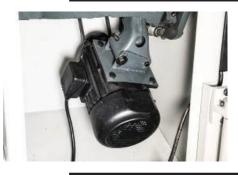
• 3HP Single phase motor with tilting capability.
