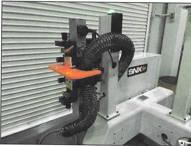
Four adjustable knobs for fine tuning trimmer
